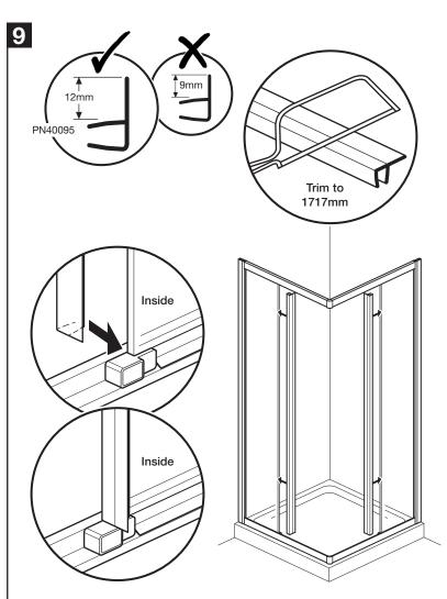
Select the vertical seals with the 12mm flipper (PN40095) and trim to 1717mm.
