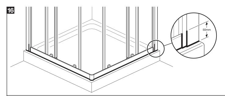
From the outside only, apply sealant to the bottom of the enclosure and 50mm up the wall channels and vertical joints as shown.
