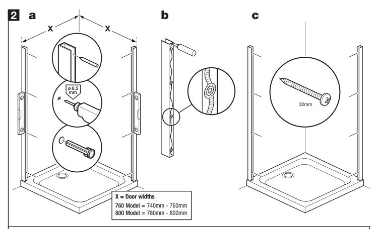
**a:** Place the wall channels on the tray ensuring they are vertical and an equal distance back from the front of the tray. Place masking tape against the wall before marking drill hole positions, this will help prevent the drill bit slipping. Drill 6.5mm holes, 30mm deep and insert the wall plugs.
