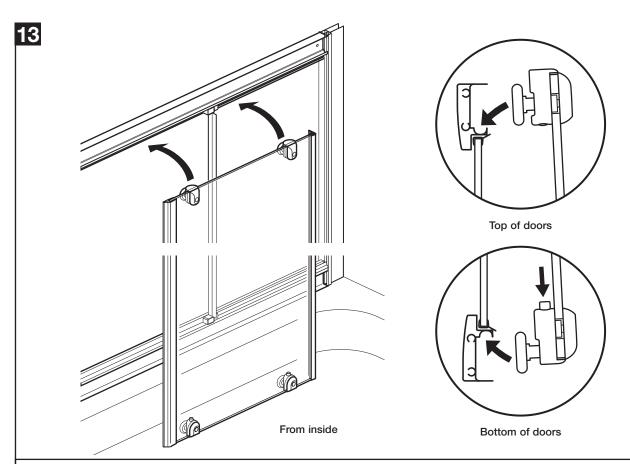
From inside the enclosure, position the top wheels into the top rail, push down the 'plungers' on both bottom wheels and position into the bottom rails.
