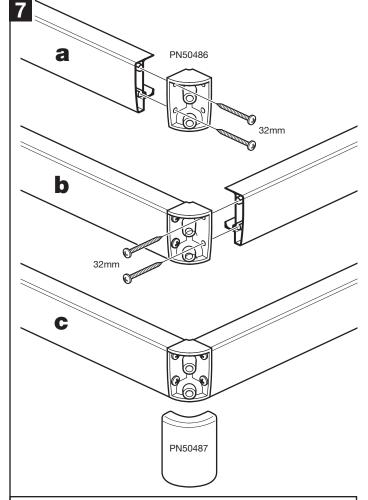
Attach the corner joints to the top and bottom horizontal rails using 32mm screws.
