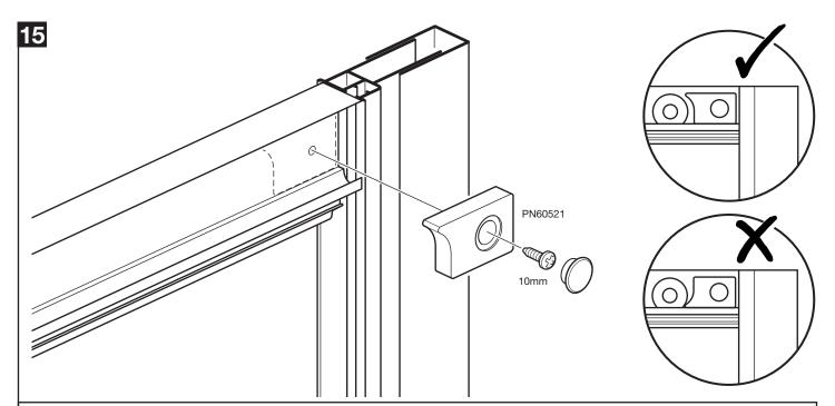
Attach 4 x bumpstops (PN60521) to the holes at the ends of the top and bottom rails using 10mm screws and screw covers. Ensure they are fitted the correct way up as shown. **Note:** If fitted incorrectly, they could cause the doors to jump out of the rail.
