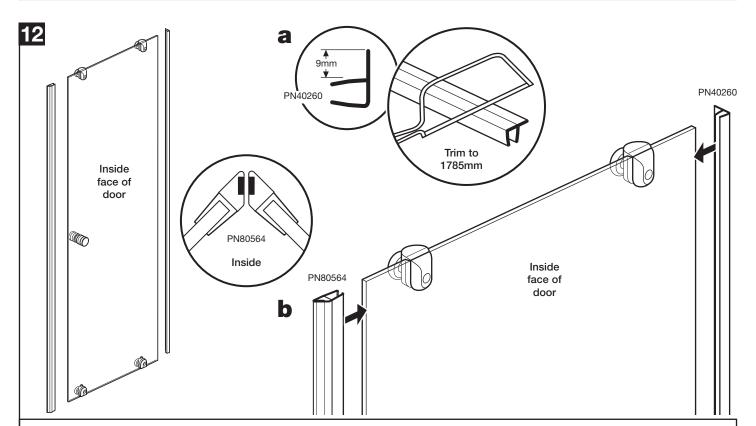
a: Select the vertical seals with the 9mm flipper (PN40260) and trim to 1785mm.
