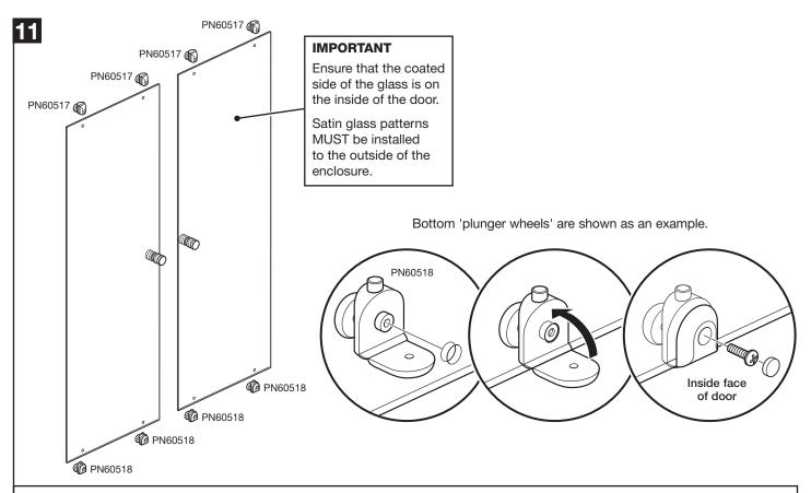
Important: Ensure that the coated side of the glass is on the inside of the door.
