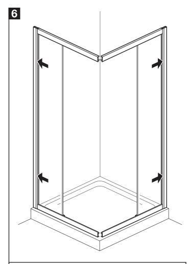
Carefully position the assembled fixed panels into the wall channels as shown.
