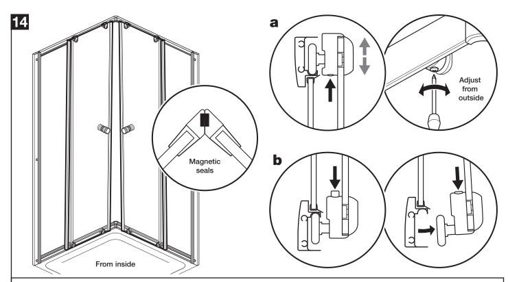
**Door adjustment:** The wheels at the top of the doors may need adjusting so that the doors slide freely and the magnetic seals meet evenly when the doors are closed.
