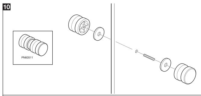
Fit the door handles to the doors ensuring the plastic washers are fitted each side of the glass.
