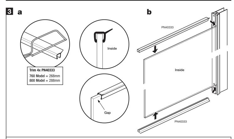
a: Trim four horizontal fixed panel seals (PN40333) to length: 760 Model = 268mm - 800 Model = 288mm.
