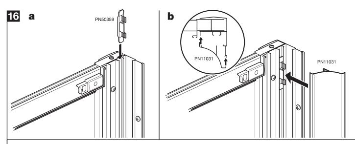
a: Insert 3 wall channel clips (PN50359) down the slot in each wall channel and space out equally down their length.
