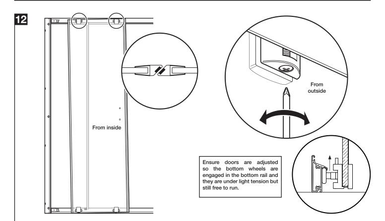
The 'wheels' at the top of the doors may need adjusting so that the doors slide freely and the magnetic seals meet evenly when the doors are closed.
