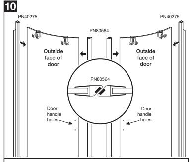
Push fit 'flipper seals' (PN40275) onto the back edge of the doors. **Ensure the flipper seal 'flaps' are on the outside of the doors.**
