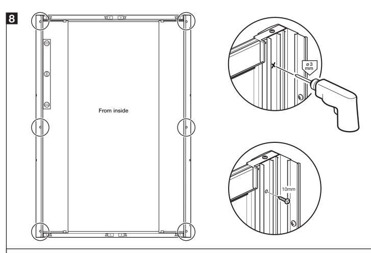
Check the door frame is vertical and is centrally positioned between the wall channels.
