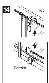
Slide the wheel cover caps (PN60490) on to the back of the wheels as shown from the inside of the enclosure.
