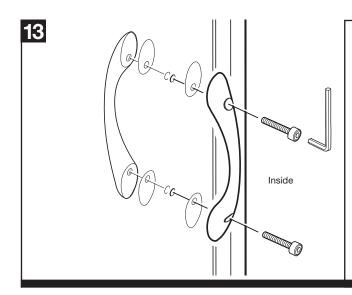
Fit the door handles to the doors with the allen bolts on the inside of the door.
