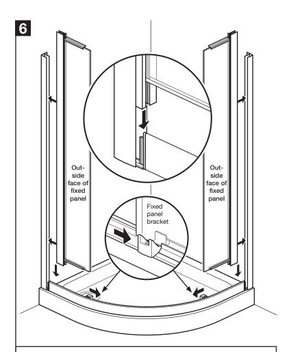
Position the fixed panels into the wall channels and slide down so that they fully slot onto the end mouldings of the bottom rail. Inside the enclosure, ensure the panels sit in the 'fixed panel brackets', slide the fixed panel brackets along the rails and position under the panels as shown.
