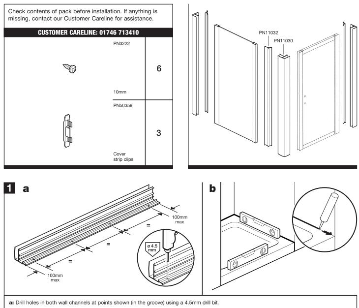
**b:** Ensure the shower tray is level in all directions. **IMPORTANT:** Clean the tray and seal the gap between the tray surface and tiles. It is important that the tray is sealed right up to the tray edge so that the bottom of the wall channel is sealed. Failure to do this will cause water to leak under the wall channel and between the tray and tiles, resulting in damp patches on the wall and under the tray.
