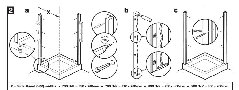
a: Place wall channels on the tray ensuring they are vertical and a minimum of 3mm back from the front of the tray. Place masking tape against the wall before marking drill hole positions, this will help prevent the drill bit slipping. Drill 6.5mm holes, 30mm deep and insert the wall plugs.
