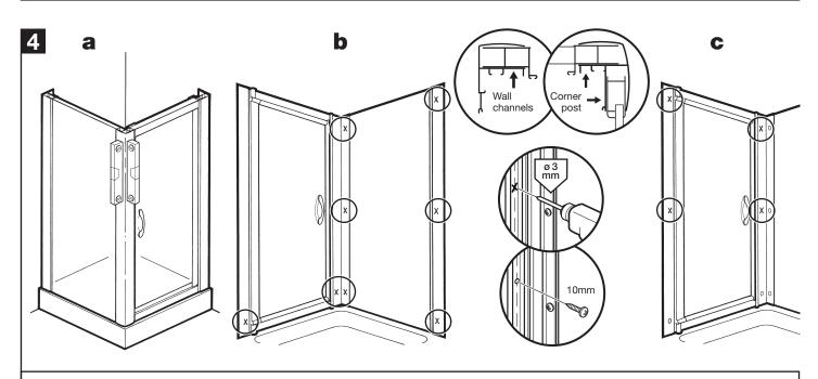
a: Check that the enclosure is vertical (see Door instruction). IMPORTANT: Ensure the door and side panel are parallel with the edge of the tray.
