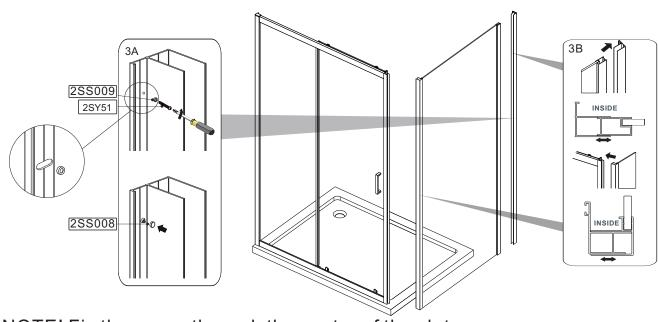
NOTE! Fix the screw through the center of the slot. This is necessary to allow enough room either side for the screw cover caps
